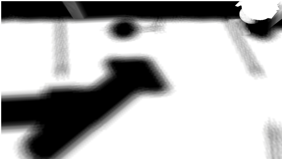
Figure 3: Shadows with 16 samples. Banding is seen because each pixel uses the same shadow map sample coordinates.
