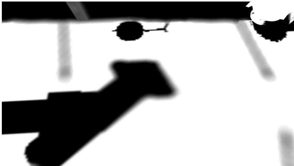
Figure 12: Soft shadows with penumbra rendered in a separate pass in lower res. Kernel scaling of 1.2 for penumbra estimation applied. Also, penumbra mask used is blurred with 7 \times 7 separable Gaussian blur with \sigma = 3 .
