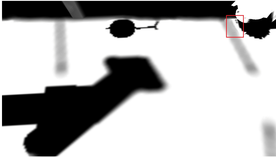
Figure 7: Regular contact-hardening soft shadows. We clearly see how far from the ground objects are. Red rectangle indicates area with shadows with highly varying penumbra size hence some jittering/jaggies can be seen. These jaggies are caused by the fact that some pixels (randomized by interleaved gradient noise) fall in areas of zero penumbra and some in areas of maximum penumbra hence varying lightness/shadowness of pixels.
