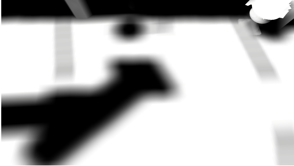
Figure 2: Naive shadows with 11 \times 11 kernel, that is 121 samples.
